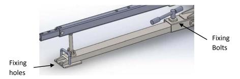
4. Secure the bottom base arms with bolts, fix the bottom base with anchors with use of fixing holes at the end of bottom base arms.
