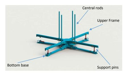
Ingoodnic uncoiling platform is made of steel and consist of two major parts: fixed bottom base and upper rotating frame. There is a bearing between the upper frame and the bottom base, which allows free rotation of the upper frame.
