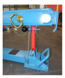
1. Set all four support pins located on the bottom base arms on vertical position and locate them into the housing places on the upper frame arms. Secure the loading pins with locking pins.
