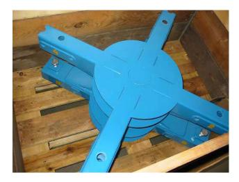
1. Put the body of uncoiling platform on the ground in a place of installation. Bars of the bottom side of the body are marked with letters: A, B, C, D. Bars of the upper side of the body are marked with numbers: 1, 2, 3, 4.
