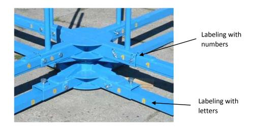
2. Assemble first the bottom base arms to the bottom part of the base according to marking with letters (A-A, B-B, C-C, D-D). Then assemble the upper frame arms to the upper part of the base according to marking with numbers (1-1, 2-2, 3-3, 4-4).
